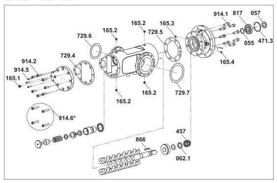
**Notice:** Only the numbered parts are included in the maintenance kit. Before installation read and observe the operating instructions of the pump/station.
