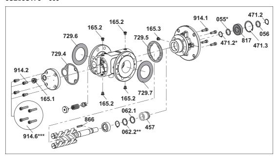
**Notice:** Only the numbered parts are included in the maintenance kit. Before installation read and observe the operating instructions of the pump/station.
