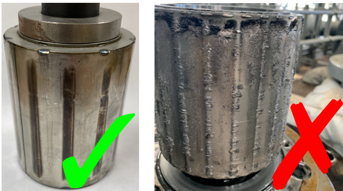
Fig. 11: Inner rotor Left: Inner rotor without adhesions Right: Large amount of iron particles accumulated on the inner rotor
