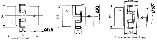
Fig. 9: Coupling alignment measuring points
