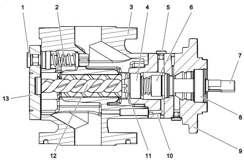
Fig. 3: Pump structure
