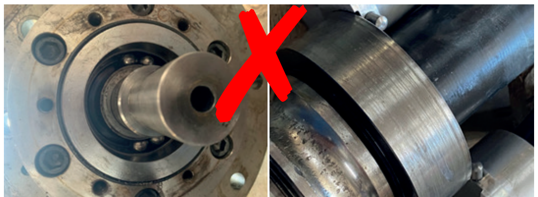
Fig. 14: Bearing Left: Worn bearing with missing cage and several rolling elements Right; running surface of bearing inner ring with embedded deposits
