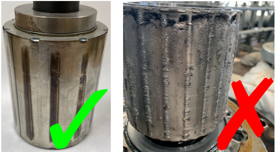
Fig. 13: Inner rotor Left: Inner rotor without adhesions Right: Large amount of iron particles accumulated on the inner rotor
