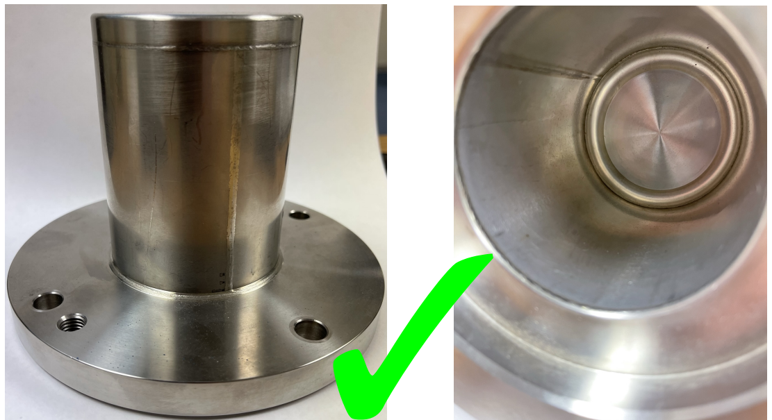
Fig. 15: Containment can Left: Outer surface free from grooves Right: Inside free from grooves
