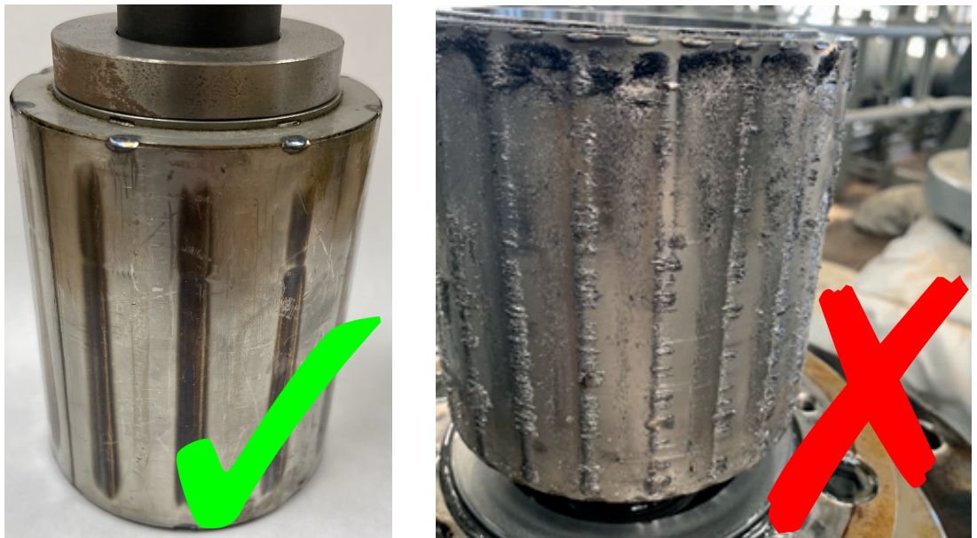
Fig. 17: Inner rotor Left: Inner rotor without adhesions Right: Large amount of iron particles accumulated on the inner rotor
