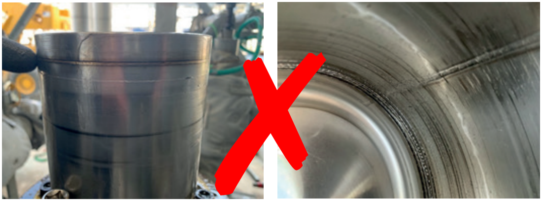
Fig. 16: Containment can Left: Groove extends over the entire wall thickness Right: several deep grooves in succession
