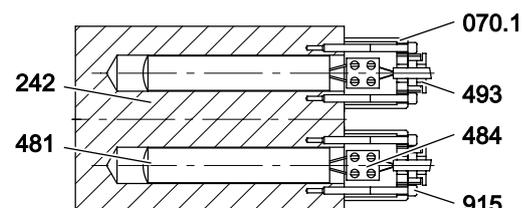
Electrical heating system for Size 370 – 880
