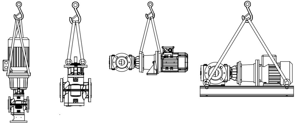
Fig. 6: Fastening of hoisting equipment - principle diagrams
