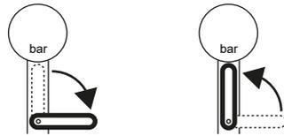
Fig. 9: Pressure gauge shut-off valves closed/open - principle diagram
