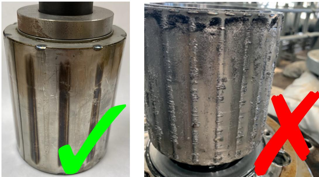
Fig. 13: Inner rotor
