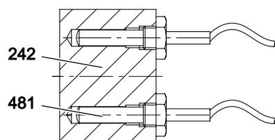
Electrical heating system for Size 5 – 42 and 235 – 275
