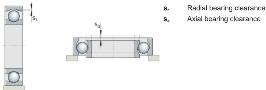
Fig. 15: Bearing clearance
