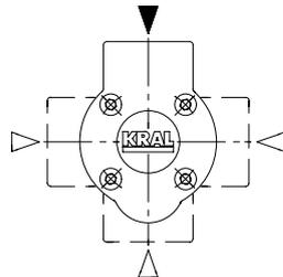
**Note** At pumps without integrated overflow valve the suction housing can be mounted with a respective rotation of 90°.
