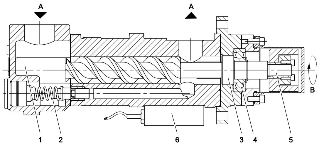
Fig. 3: Pump structure
