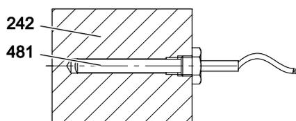
Electrical heating system for Size 55 – 210
