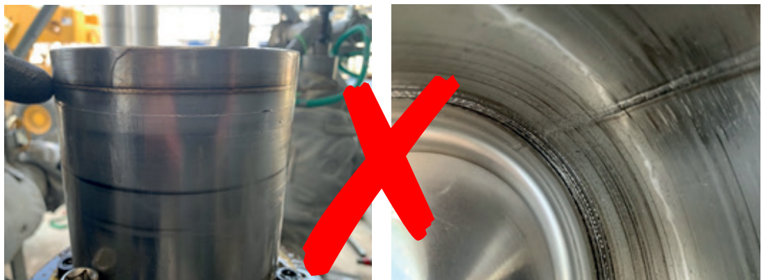
Fig. 10: Containment can Left: Groove extends over the entire wall thickness Right: several deep grooves in succession
