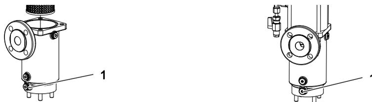
Fig. 16: Strainer (left) / Deaerator with integrated strainer (right)
