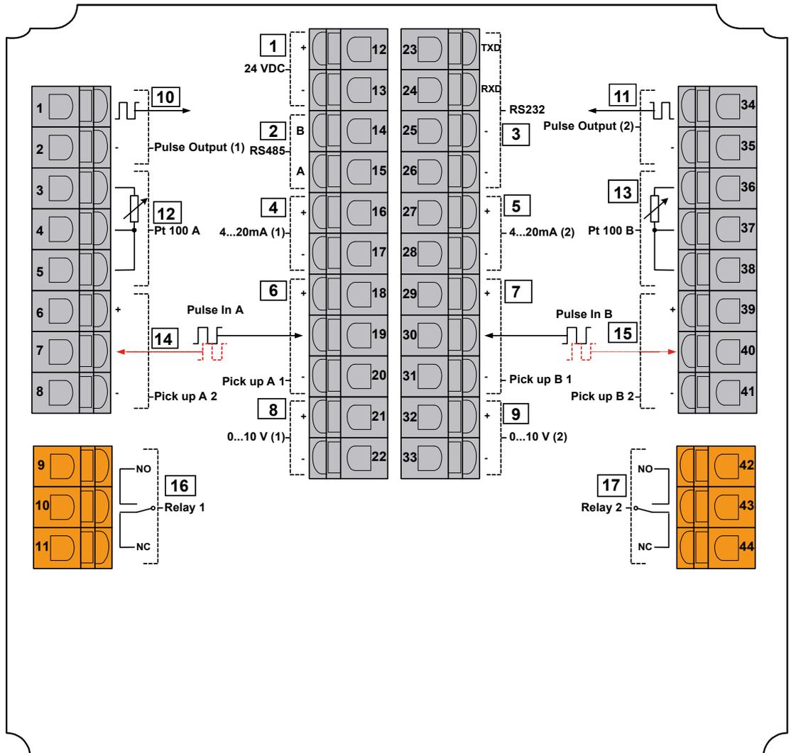
Fig. 2: Termination panel electronic unit
