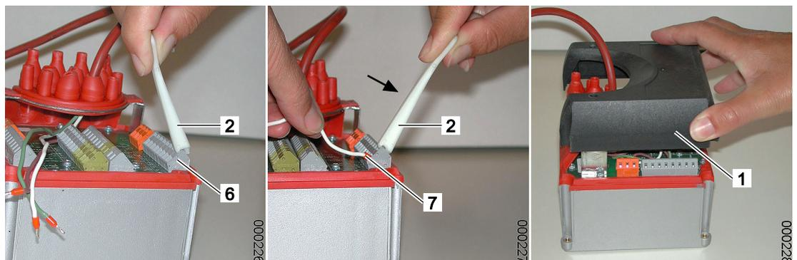
4. ▶ Hook the short arbour of the terminal tool 2 into the tension spring terminal 6 and press away from the cable opening so that the cable opening opens.
