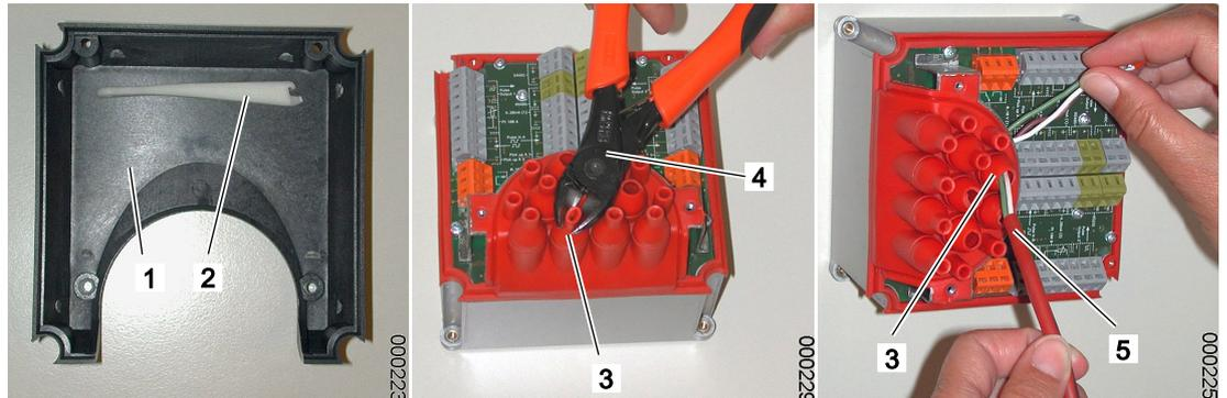
1. ▶ Remove the rear device cover 1 and remove the terminal tool 2.
